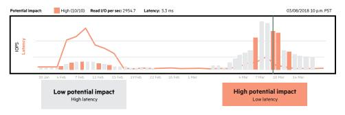
Figure 5. Historical IOPS activity with potential impact reflected in orange color and a numerical latency severity score
